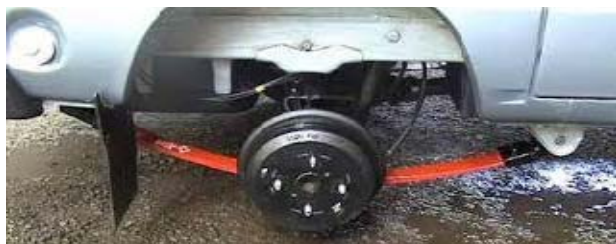
Fig. 1.2: Leaf Spring Used In Maruti Omni
